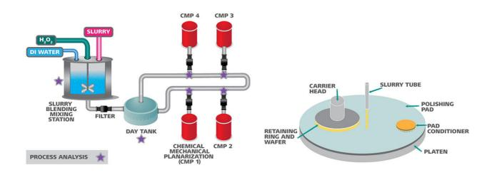
Figure 1. (Left) A typical Chemical Mechanical Planarization (CMP) process. (Right) Top view of a CMP polisher.
