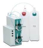
The version for voltammetry is equipped with the complete accessories for the automatic rinsing and emptying of the measuring vessel.
