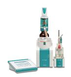
Coulometric titrations are carried out easily and quickly with the **851 Titrando**.
