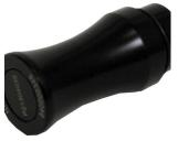
Lab grade fiber optic Raman probe assembly for cut-on start from 65 cm  $^{-1}$  with hand trigger; 105 µm diameter, 0.22 NA fiber for 785 nm excitation, 200 µm diameter, 0.22 NA for Raman pickup. Optical density >6; 1.5 m fiber length terminated in SMA905 on the spectrometer end and FC/PC on the laser end. Adhesive sealed quartz window for noncontact sampling. 5.4 mm working distance. Not for immersive use.
