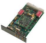
In the Bipotentiostat mode, a fixed potential is applied to the second channel (second Working Electrode) while applying a potential step or a sweep to the first channel (first Working Electrode). In the Scanning Bipotentiostat mode, a potential offset with respect to the first channel is applied to the second channel.
