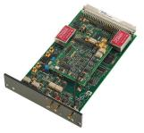
Measurements in the sub  $\mu g/cm2$  are possible. The EQCM can be fitted with 6 MHz, AT-cut crystals.
