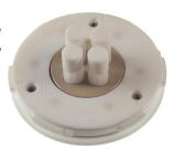
Titration head with 3 NS14 and 4x 6.4 mm openings for using 120 mL beakers in Pick&Place modules of the OMNIS Sample Robot Pick&Place with two retracted dosing tips. Prepared for being equipped with rinsing and aspiration tubing.
