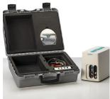
The BA is a dual-mode bipotentiostat module that converts the Autolab into a double channel potentiostat with which measurements on 2 working electrodes can be performed sharing the same counter and reference electrode.
