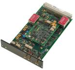
Measurements in the sub  $\mu g/cm2$  are possible. The EQCM can be fitted with 6 MHz, AT-cut crystals.
