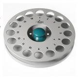
Sample rack for 810 Sample Processor, 814 USB Sample Processor, 855 Robotic Titrosampler "Light" suitable for 21 sample vessels. The following sample vessels can be used: 100 mL digestion tubes (CSB).
