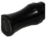
Lab grade fiber optic Raman probe assembly for cut-on start from 65 cm $^{-1}$  with hand trigger; 105  $\mu$ m diameter, 0.22 NA fiber for 785 nm excitation, 200  $\mu$ m diameter, 0.22 NA for Raman pickup. Optical density >6; 1.5 m fiber length terminated in SMA905 on the spectrometer end and FC/PC on the laser end. Adhesive sealed quartz window for non-contact sampling. 5.4 mm working distance. Not for immersive use.
