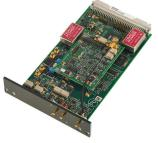
The MUX module series allows you to perform electrochemical experiments on multiple cells or multiple working electrodes, sequentially. The cell to perform measurement on can be selected either manually or automatically using the sequencing option of NOVA. Metrohm Autolab offers two types of MUX modules.
