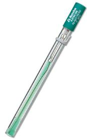
The ground-joint diaphragm, which is insensitive to contamination, offers a constant and reproducible electrolyte outflow. Additionally, the reference electrolyte is gelled for even better signal stability. The sensor is delivered with  $c(KCl) = 3 \text{ mol/L}$  as bridge electrolyte, which can be freely selected and exchanged as needed.
