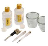
6.5339.060 CVS electrode equipment with 2 mm platinum electrode for Professional VA/CVS instruments for intensive use
