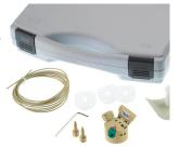
Equipment comprised of Wall-Jet cell with additional accessories. For carbohydrate analysis with a gold working electrode and a Pd reference electrode.
