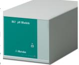
The pH Module has two USB interfaces for connecting printers, barcode readers or sample changers and four MSB interfaces for stirrers or Dosinos (for the addition of auxiliary solutions or for standard addition). Both in conjunction with the Touch Control and also integrated in *tiamo* ™ full (from 2.0), it is in compliance with GLP and FDA 21 CFR part 11 requirements.
