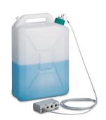
The metal-free sensor works in solutions with very low conductivity. Therefore it may be used in ion chromatography.
