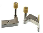
The cable cover protects the MDL and Ethernet cables connectors on the OMNIS Sample Robot.
