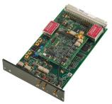
With this module it is easy to separate the capacitive current from the faradaic current. In addition the integrator is effective in reducing signal noise by averaging it out.
