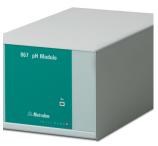
The pH Module has two USB interfaces for connecting printers, barcode readers or sample changers and four MSB interfaces for stirrers or Dosinos (for the addition of auxiliary solutions or for standard addition). For use with OMNIS Software, tiamo software, or Touch Control unit. Compliance with GMP/GLP and FDA regulations such as 21 CFR Part 11, if required.
