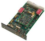
With this module it is easy to separate the capacitive current from the faradaic current. In addition the integrator is effective in reducing signal noise by averaging it out.
