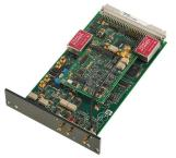
The pX1000 module can also be used as an additional differential electrometer, with the same specifications as the main Autolab electrometer. The pX1000 module is compatible with the Metrohm pH and temperature sensors.
