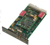
The ECD module provides 2 additional current ranges of 1 nA and 100 pA giving a minimum current resolution of 0.3 fA. The ECD module also has a built in third order Sallen-Key filter, with 3 RC-time constants that help to filter out noise.
