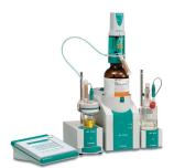
Recommended coulometry measuring range: 10  $\mu g$  - 200 mg absolute water
