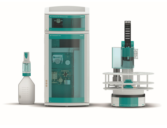
Figure 1. Instrumental setup including a 940 Professional IC Vario (center), 947 Professional UV/VIS Detector Vario SW (top center), 858 Professional Sample Processor (right), and MiPCT-ME, performed with the Metrosep A PCC 2 HC/4.0 and a Dosino (left).
