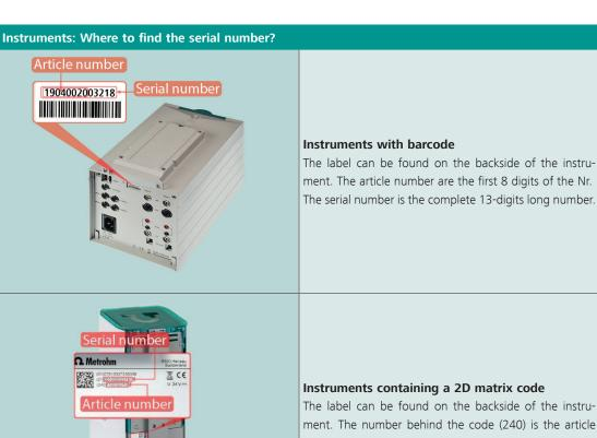
The label can be found on the backside of the instrument. The number behind the code (240) is the article number, the number behind (21) is the serial number.
