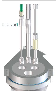
1 Insert the buret tip 6.1543.200 of the dosing unit into the remaining opening at the rear on the vessel lid.
