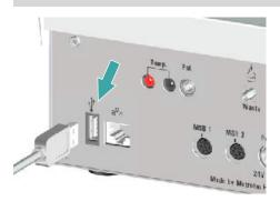
A printer can be connected directly to the USB connector (Type A) (with a 6.2151.020 connecting cable ), as can a USB keyboard, a barcode reader or a USB flash drive (for storing and loading methods, etc.).
