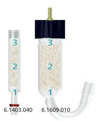
1 Insert a small cotton plug into the bottom of the two adsorber tubes.
