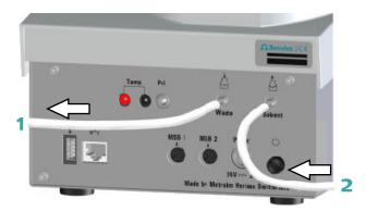
Take care to ensure that you connect the tubings to the pump correctly. Proceed as follows:
