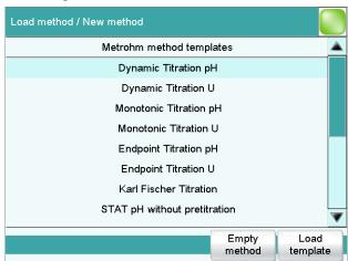
Select the template Dynamic Titration pH and tap on [Load template].
