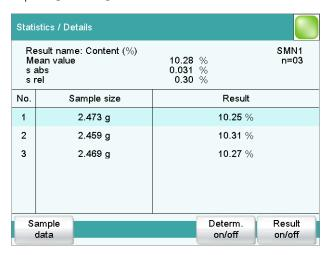
In the upper part of the display you will see the mean value of the result as well as the absolute and the relative standard deviation. The single results of the titrations are listed in a table.
