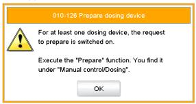
All tubings and the cylinder of the buret are rinsed with the **Prepare** function. The preparing of the buret unit is described in *chapter 3.3.1, page 25*. The buret unit must, however, first be configured (see chapter 2.2.5, page 9).
