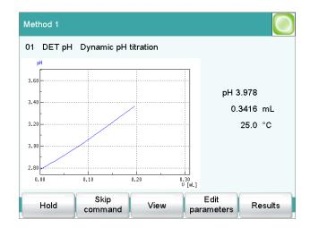
Use the [ ] key to move to the main page while a determination is running. It is thus possible to modify individual parameters during a determination. However, only those parameters which do not decisively influence the running determination can be modified. Use the [Live display] button in the main dialog to switch back to the "Live" depiction of the determination.
