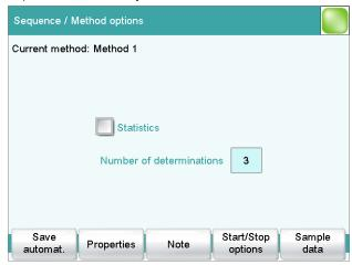
Here you can define the statistics function for this method. You can specify the number of determinations for which the respective statistical calculations are to be carried out.
