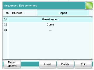
Two reports are already specified. According to these parameters, a result report and a titration curve will be printed out automatically after each determination.
