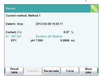
Result name and result are displayed. Furthermore, the measured value and volume of the endpoints found are displayed.
