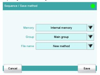
You can save the method in the instrument's internal memory, on a USB storage medium or in a shared data directory in a network. In addition, you can also create different groups and/or folders for the methods.
