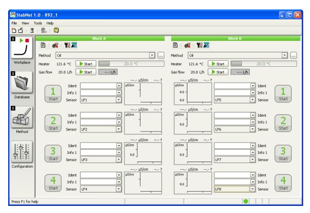
Because the **Conductivity sensor assignment** parameter is enabled for this method, the **Sensor** field also appears for each measuring position. The conductivity sensor used for the respective position has to be selected in this field. All of the conductivity sensors defined in the configuration are available for selection.
