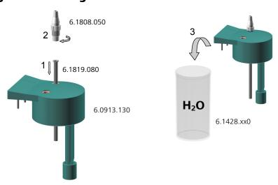
Proceed as follows to mount the measuring vessel cover:
