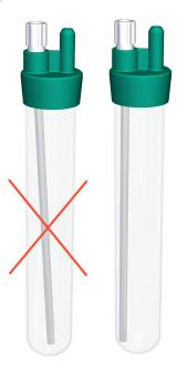
Place the prepared reaction vessel in the 6.2041.190 reaction vessel holder.
