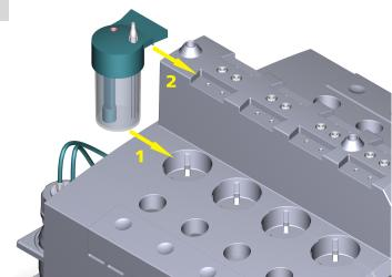
Insert the measuring vessel into the opening (1) provided for this purpose in the instrument. While doing so, carefully guide the connector plug for the measuring vessel cover into the electrode connector (2).
