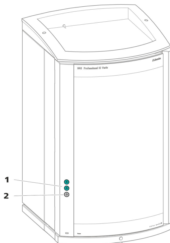
Figure 3 Feed-throughs on the door
