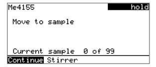
The method run is interrupted. However, currently running movements of the sample rack or the lift will be finished.
