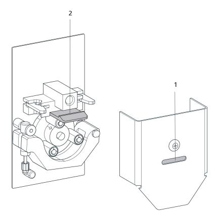
2 Attach contact pin (1) on the safety shield onto the opening (2) of the sensor.
