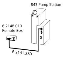
Figure 11 Remote connection Remote Box — 843
