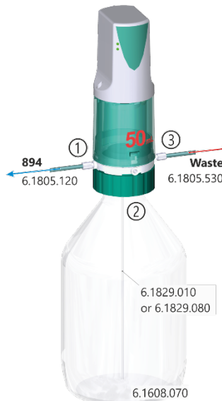
Figure 5. Setup of tubing connections of the 50 mL dosing unit used for the addition of e.g., VMS.
