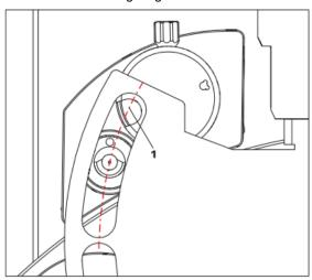
When you have found the correct position, please tighten the screw to secure the LQH Station completely to the Sample Processor.
