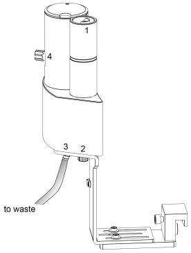
Number 4 in the picture above shows the attachment point of a capillary in case of a dilution feature and number 1 indicates the rinsing entity.
