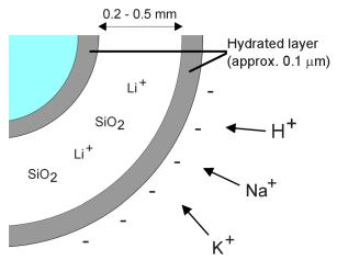
Cross-section of a pH glass membrane. If several cations are contained in the measuring solution, then these will compete for the free spaces in the hydrated layer. Potassium and sodium in particular can form deposits in the glass membrane, thus leading to longer response times.
