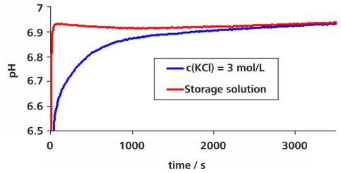
pH measurement in NaHCO $_3$  0.05 mmol/L. An Aquatrode glass stored in the storage solution exhibits a considerably shorter response time than an electrode glass of the same type stored in KCl for the same period of time.
