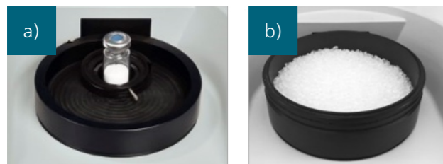
Figure 2. Solid sample placement for NIR spectra measurement. a) Direct measurement of powder substance in a vial. b) Large heterogeneous samples can be analyzed using large sample cups.
