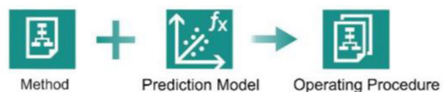
Figure 10. Structure of operating procedures in Vision Air. An operating procedure defining how a measurement is done consists of prediction models and a method which specifies different measurement parameters.
