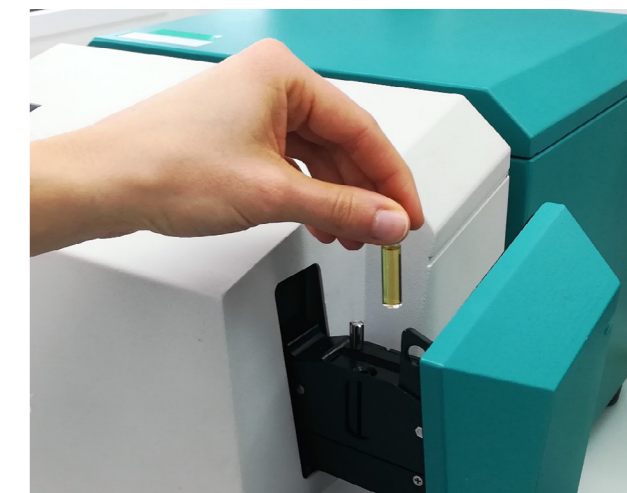
Figure 1. XDS RapidLiquid Analyzer and a polyol sample present in a 4 mm disposable vial.
