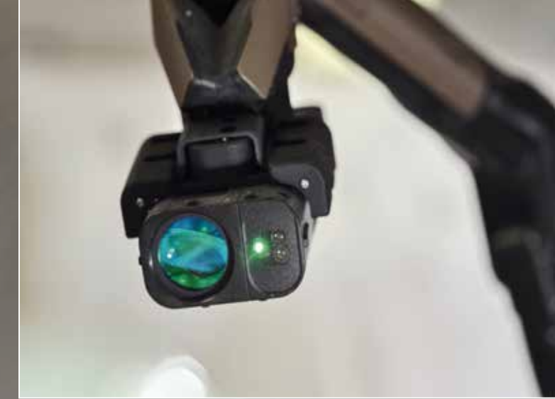
Identify unknown chemicals from a distance: MIRA XTR DS with the Autofocus Standoff Attachment deployed with the IBEX CBRNE robot.
