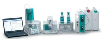
MVA-3 is the optimal 797 VA Computrace system for fully automated trace analysis. One or two parameters can be determined in small series of up to 18 samples. The samples are placed on the sample rack of the 863 Compact Autosampler. Transfer and analysis of the samples takes place automatically, controlled by the software of the 797 VA Computrace.
