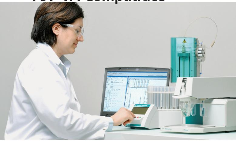
The all-round instrument for voltammetry
