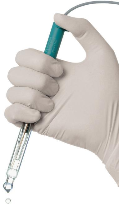
**Easy cleaning of the diaphragm:** Just press once on the electrode head and the electrolyte flows out. The diaphragm does not need to be touched any more for cleaning.
