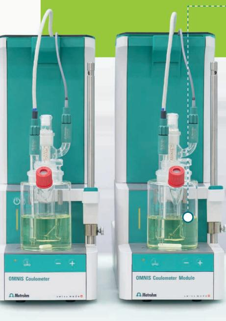
Coulometer, this can no longer happen. The system recognizes the addition of the sample and starts the titration automatically.
