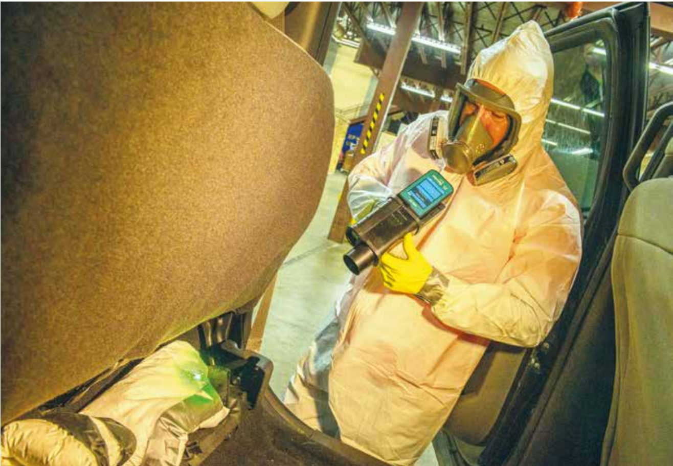
MIRA XTR DS enables the contact-free and safe determination of chemicals and hazardous substances.
