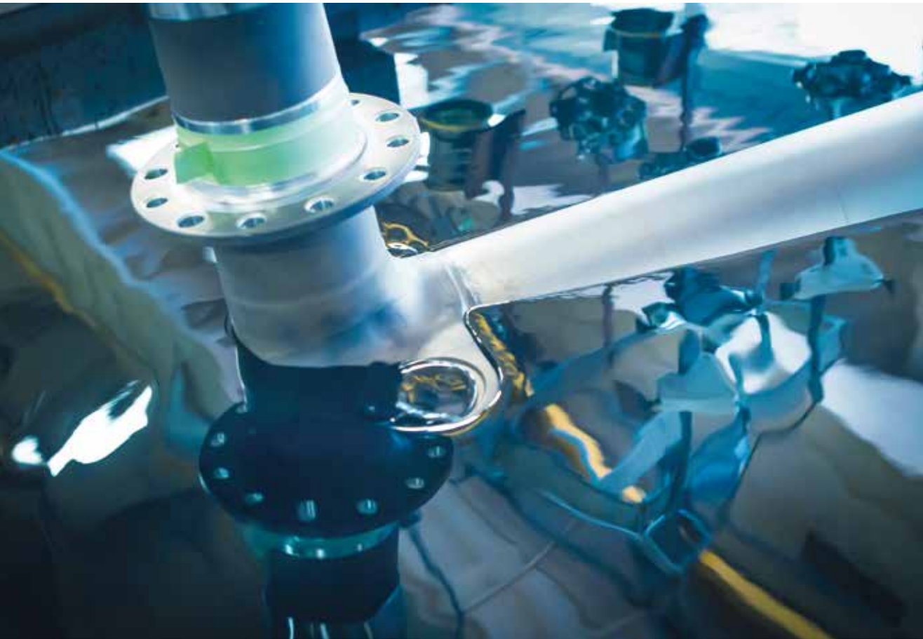
Electroplating protects against corrosion and thus ensures safe operation – here, of an airplane nose landing gear
