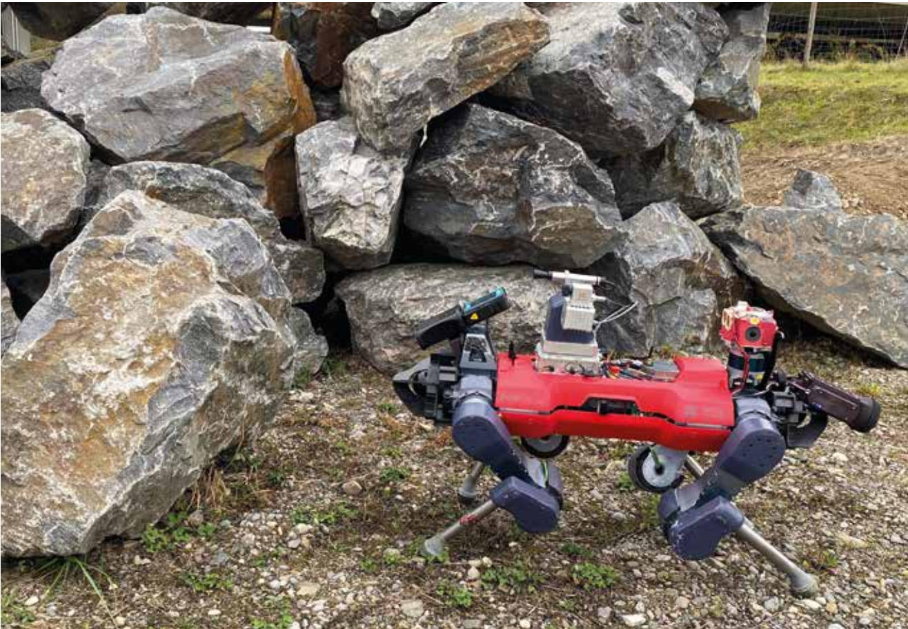
Explosives search in rough terrain: MIRA XTR DS in use with the quadrupedal robot from ANYbotics.
