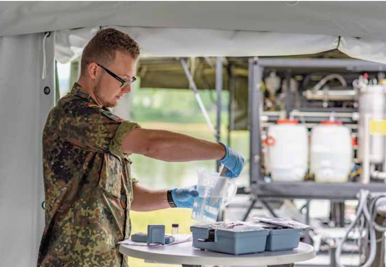
pH and conductivity measurement in the field. Photo: German Armed Forces
