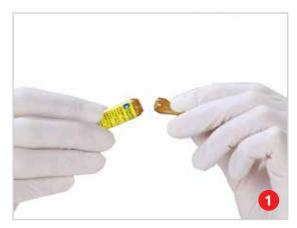
Carefully break open the ampoule of Heroin standard by snapping off at the neck. Using the dropper, transfer contents into the sample vial.
