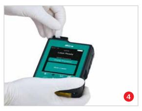
Insert colored end of the SERS test strip into the slot on the attachment with colored side facing the instrument, stopping when resistance is met.
