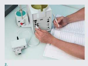
Proper signal transmission via various **communication interfaces** (USB, MSB, ...) is essential to the reliable operation of the system as a whole. This functionality is checked with specially developed test adapters with the associated testing software.
