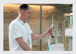
The exact dosing of liquids is a critical factor in titrations. A high-precision dosing drive is responsible for ensuring accuracy. A **special spindle measuring device and a calibrated gauge** are used to make an exact check of the accuracy of the drive.
