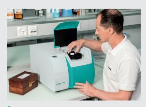
In optical measurement systems such as NIR spectrometers, measurement quality is highly dependent on **wavelength accuracy and photometric stability**. To ensure precision, the instruments are calibrated using **certified reference standards**.
