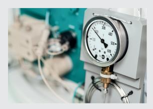
Along with the column and the detector, the quality of an ion chromatographic measurement depends on the proper functioning of pumps. Key indicators are pressure accuracy, pressure stability, and a pressure integrity test (leak test).
