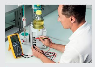
An important test performed at the very beginning is the **Safety Check**. This entails using a multimeter to check the safety of the electrical connection.
